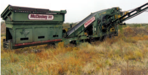
MCCLOSKEY Turbo Wheel Mounted Vib. Screen
