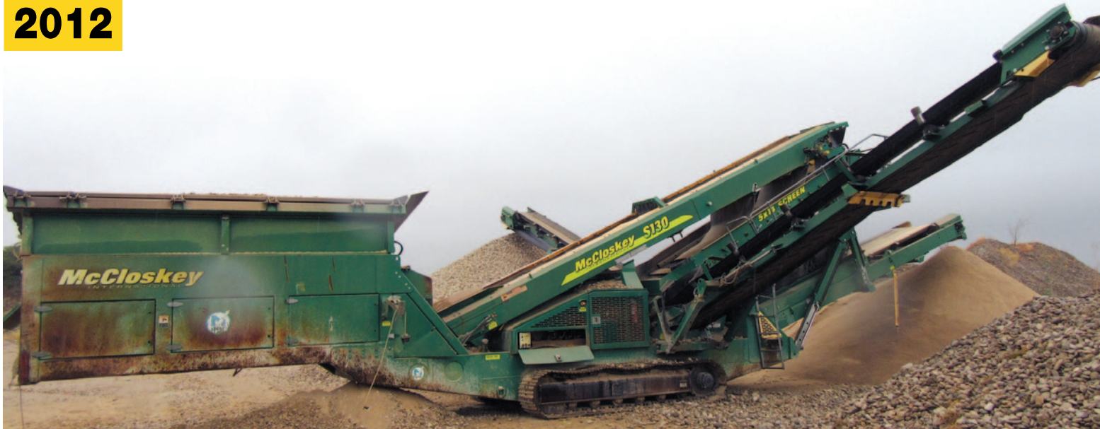
MCCLOSKEY S130 Crawler Mounted Vibratory Screen
