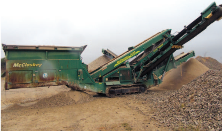
MCCLOSKEY S130 Crawler Mounted Vibratory Screen
