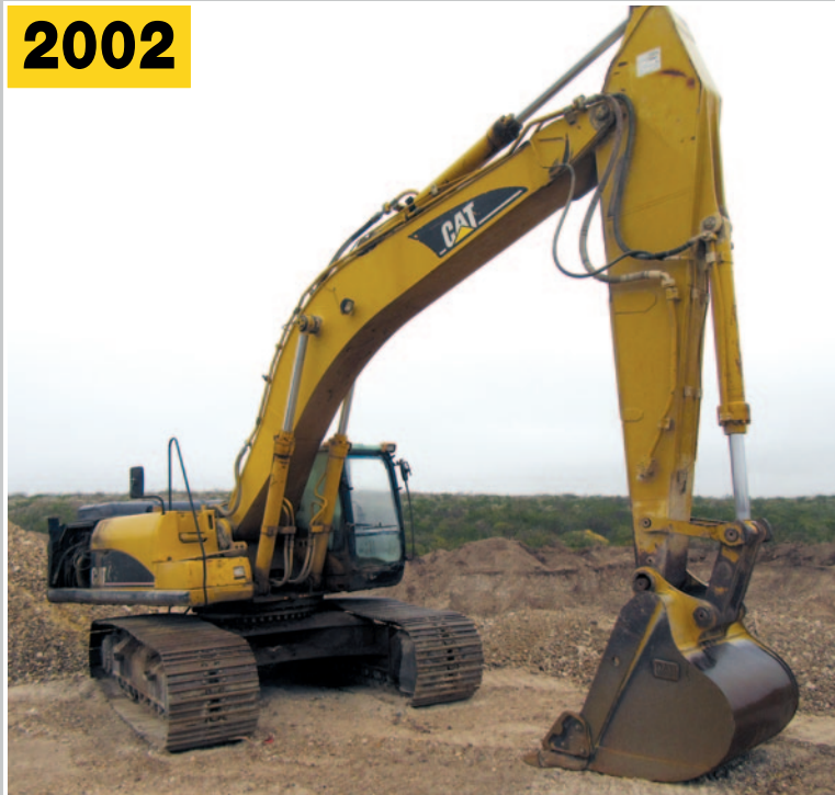
CAT 330CL Crawler Mounted Hyd. Excavator
