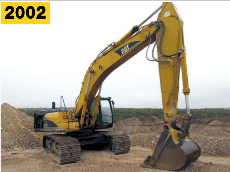
CAT 330CL Crawler Mounted Hyd. Excavator
