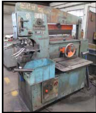
Scotchman 6509-24M 65 Ton Hydraulic Ironworker
