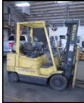
Hyster S50XM 4500 Lb Cap LPG Forklift
