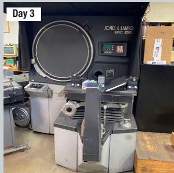
Jones & Lamson Epic 230 Clean Room Optical Comparator with DRO
