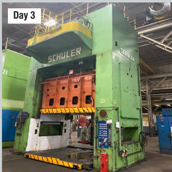
500 Ton Schuler SSSC Press, 141" x 96" Ba, Windows, Rolling Bolster
