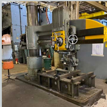
8' x 19" Col. Carlton Radial Arm Drill with Extended Base
