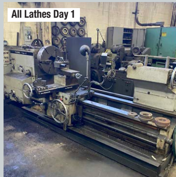
40" Clausing Trident 40" x 72" Geared Lathe
