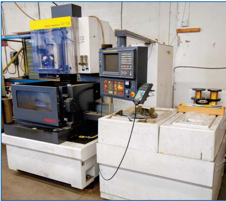
FANUC ROBOCUT ALPHA-1B WIRE EDM
