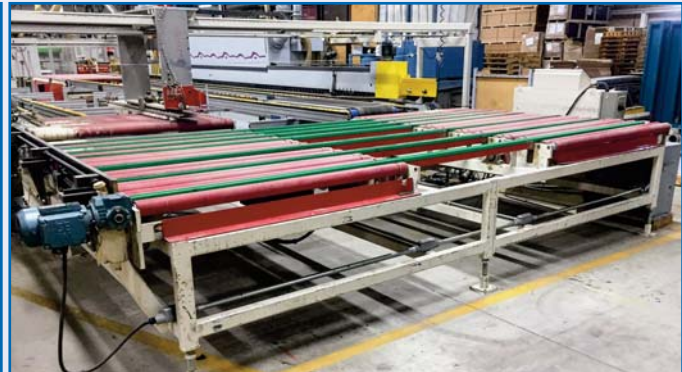
DEFIANCE 0201 CROSS TRANSFER CONVEYOR SYSTEM
