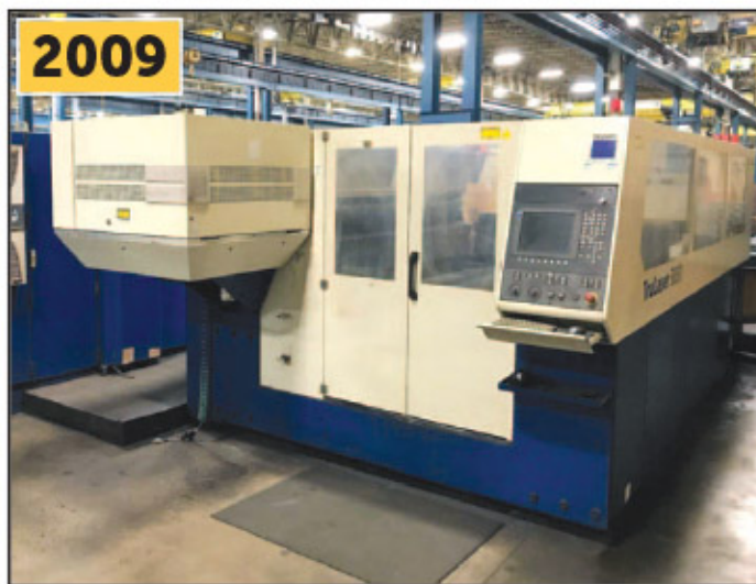
Trumpf TruLaser 3030 CNC Laser Cutter
