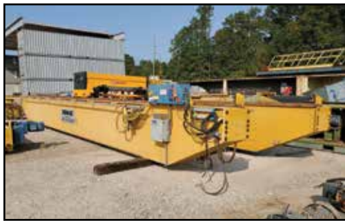
DEMAG 40-Ton x 46' Span Double Girder Bridge Crane w/KONE Wire Rope Hoist
