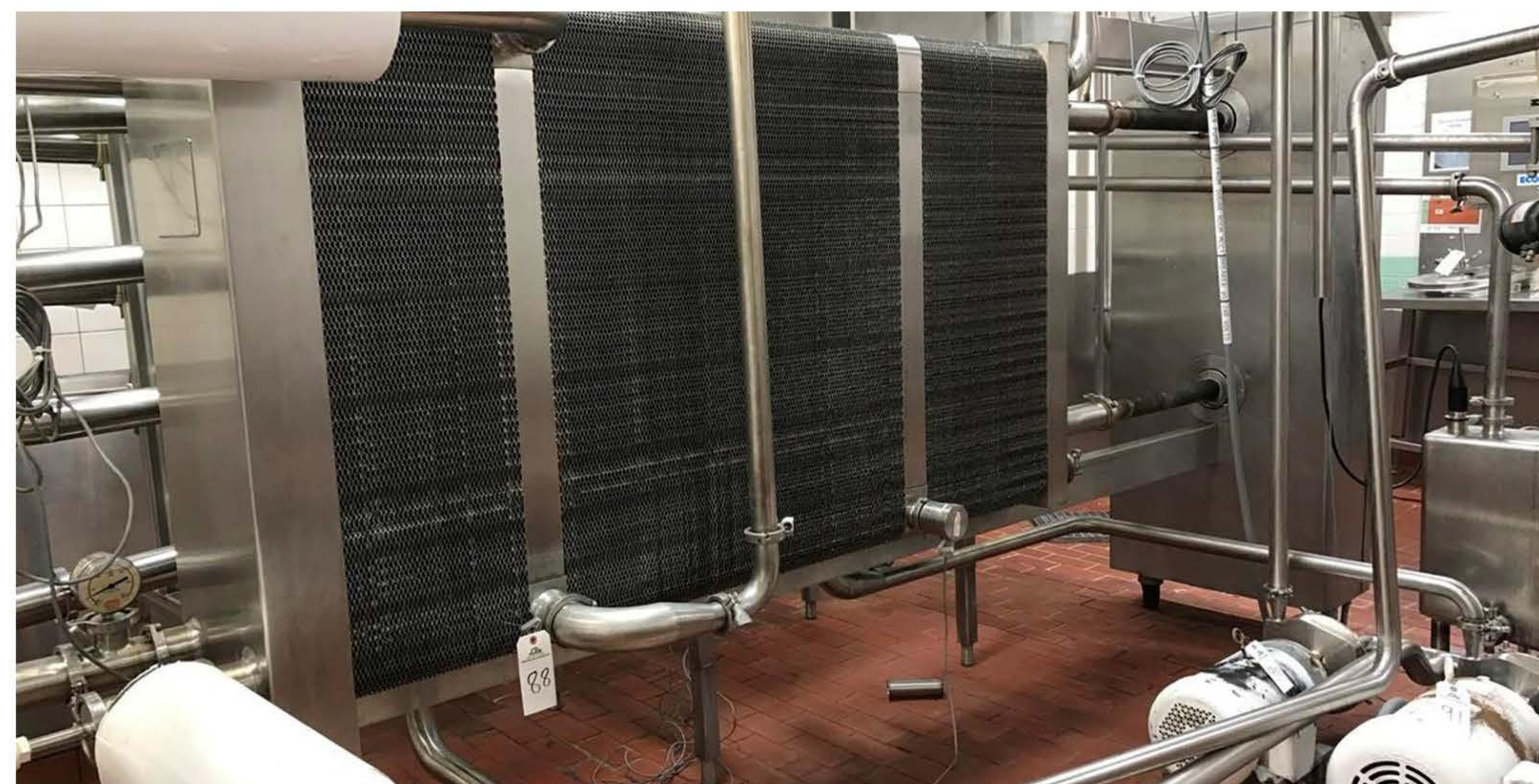
HTST WITH APV MODEL CR30 HYDRAULIC PLATE AND FRAME HEAT EXCHANGER
