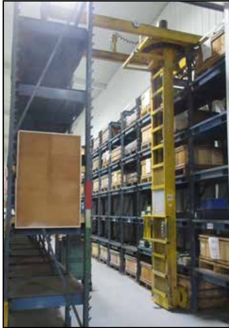
2,000 LB STORAGE/RETRIEVAL CRANE & RACKING SYSTEM
