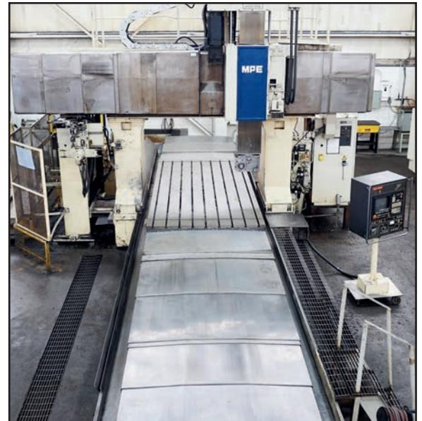
TOSHIBA SHIBAURA MPE-2140 CNC 5 FACE GANTRY MILL
