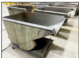
VIEW OF DUMPING HOPPERS
