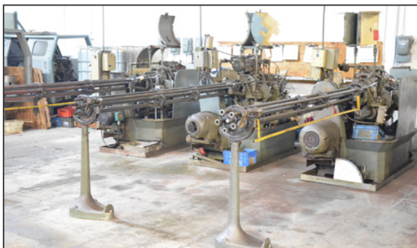
Partial view of DAVENPORT universal automatic screw machines available
