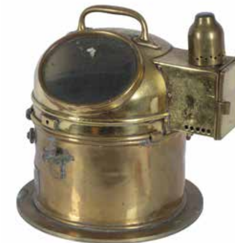
185 A ships compass in polished brass cylindrical case, with large handle to top. Spirit burner and label 'Patt 0183. No 18472.H'. Diameter 24cm.
