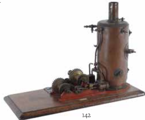
142 A period model of a winding engine, with drums and driven by a twin cylinder engine linked to vertical copper boiler.
