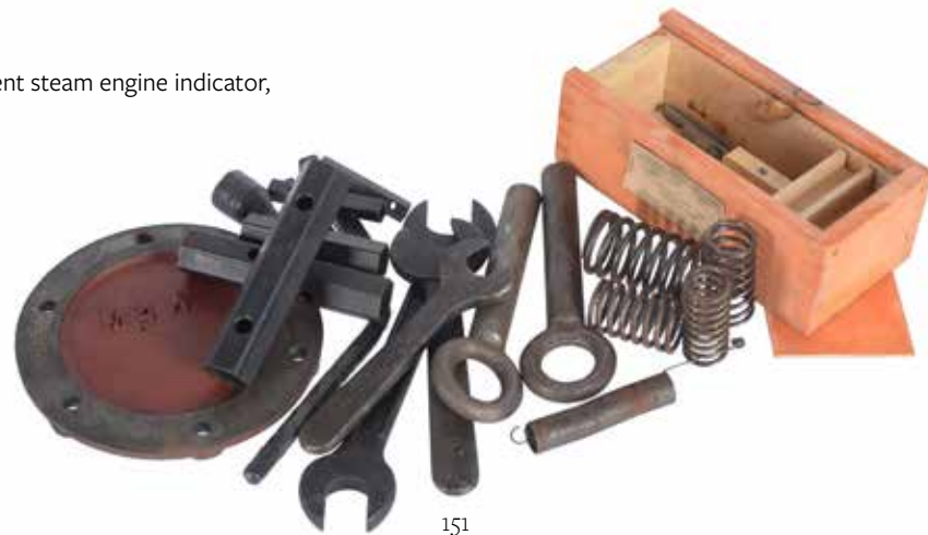
151 An original Gardner tool box with contents. Circa 1960. To include M4a cylinder cover, pair of engine lifting pins, three wrenches and seven box wrenches.
