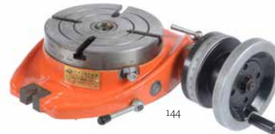
144 A Chester UK rotary milling table, of 16cm diameter with locking levers, cast iron base and graduated divisions and handle. Base 28cm by 23cm excluding graduation head. (Unused)
