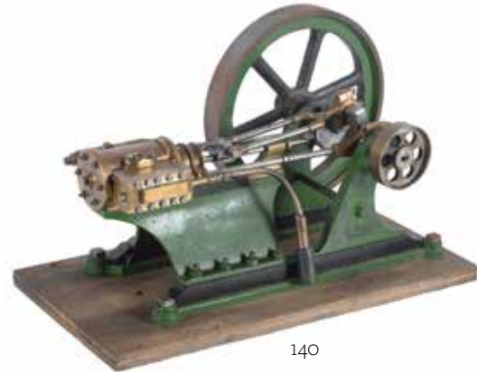
140 A vintage model of a horizontal mill/wall engine, having eccentric driven pistol steam valves, open crank with oiler cups, 16cm diameter, spoked flywheel and mounted on wooden plinth.
