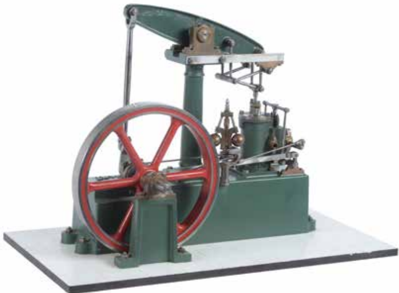
80 A Stuart Turner live steam beam engine, the turned central column supporting beam with split gun-metal bearings, Watt's parallel motion, single cylinder 1 inch bore by 2 inch stroke with fitted outside steam valve operated from eccentric mounted on the open crank with 7 inch diameter spoked flywheel and rope wheel to crank with rope driving speed governor with shut off linkage to steam inlet. The model finished in green and red paintwork and mounted on simulated tile plinth. Plinth length 43cm. Depth 22cm. Total height 29cm.
