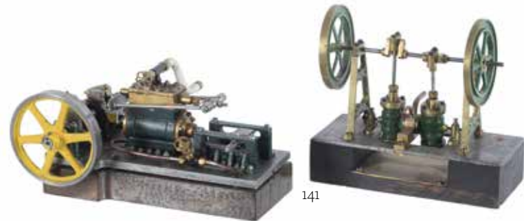
141 A small horizontal mill engine with central mounted cylinder, cross-head guides, balanced crank, eccentric driven steam valve and steam inlet control valve. Also a model of an over-type oscillating steam engine. Mill engine 22cm by 14.5cm.
