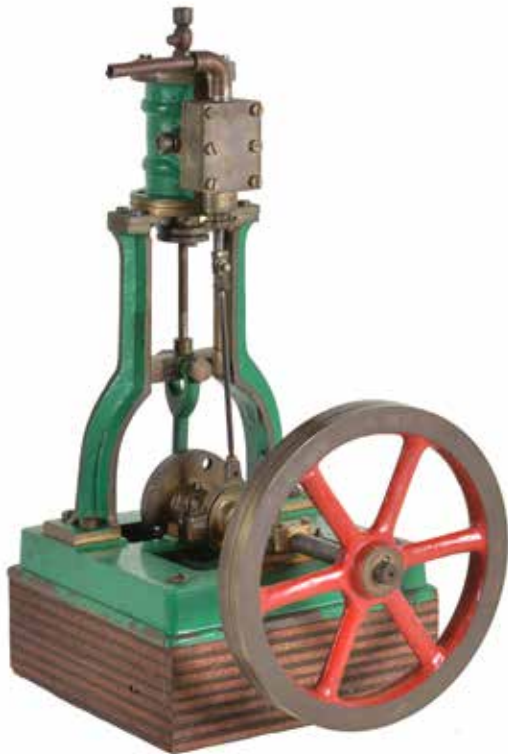
77 A rare and early Stevenson dockyard model of a live steam vertical mill engine, the single cylinder with mounted steam chest having eccentric driven steam valve with 15cm diameter flywheel. The model set on painted brass sole plate with wooden plinth. Overall height 34cm. Base 15cm by 15cm.
