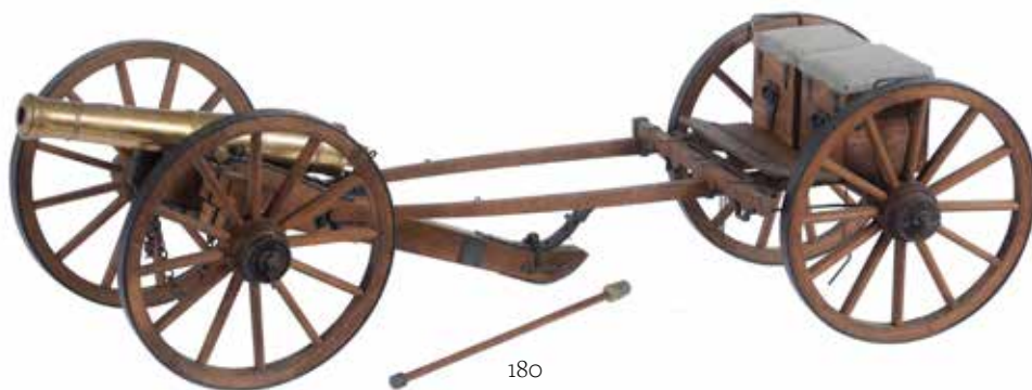
180 A hand-built model of a Napoleonic canon, having ram rod wooden spoked wheels and metal wheel rims. Built from a Bassett-Lowke kit and comes with a drivers carriage having box seats containing bucket and drag shoe. Overall length 70cm.
