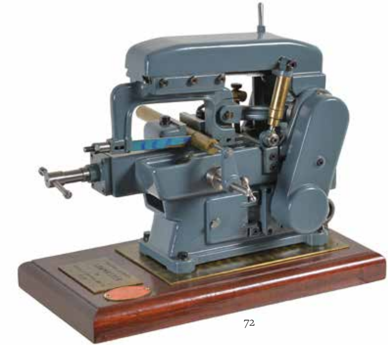
72 A very fine engineered exhibition standard model of a 1/5th scale Qualters & Smith ‘Sawmaster’ 6 inch power hacksaw, built by Barry Jordan in 1999, from catalogue reference. The model is 8 inches high.
