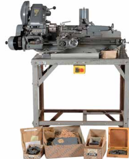
145 A full size Myford Super 7b metal working lathe, on non-commercial bench with fitted gear box, 4 inch self centre chuck, tools post, face plates, vertical slide and sundry other items.
