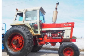
III 1466 Royal Cab, SN 18418 540/1000 pto, DR, 3-pt., TA, 20.8-38's (20%) w/dual hubs, 1 set of rear weights, tractor is very straight & original from grill to paint. Tractor has been updated w/LED lights and has most all electrical wiring refurbished, along with a past OIL Meter shows 2234 hrs., but actual are much higher.
