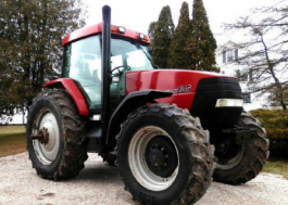
CHI MX 135 Cab MFWD Tractor, SN 86348, 16-sp. PQ W/1H Reverser, TR, Rear 3-pt. control, 540/1000 shafts, 14.9R-30's (75%) w/fenders, 480/80R 42's (70%). Tractor has had recent 58000 in electronic & tranny work. 11,761 hrs are from many hours on TMR mixer.
