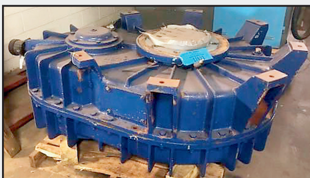
B & P Mdl. 84700 100B 250HP Muller Gear Box, Rebuilt by IDC
