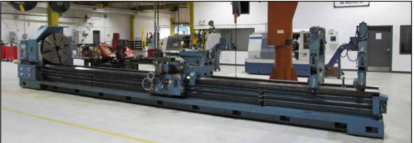
GEMINIS 43" X 309" ENGINE LATHE
