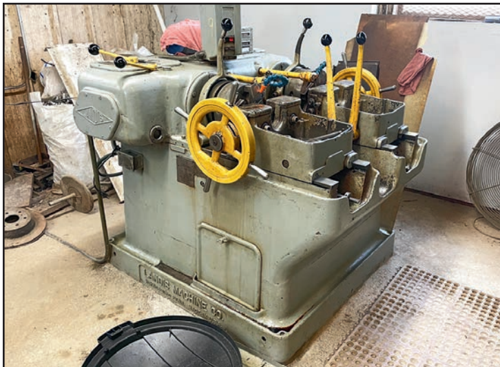
1-1/4" Landis Double Spindle Pipe and Nipple Machine, S/N UNK, (2) 1-1/4" Lanco die heads 10T, S/N T00001-900450-2, S/N 10TSR710, reamer tube and rods
