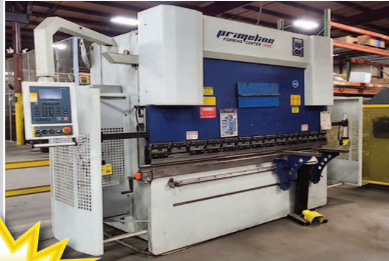
Primline Hydraulic Press Brake
