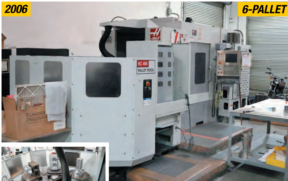
2006 HAAS EC400-6PP, HAAS CONTROL, FULL 4TH AXIS, 70 TOOL ATC, COOLANT THROUGH SPINDLE, 12,000 RPM SPINDLE, 40 TAPER
