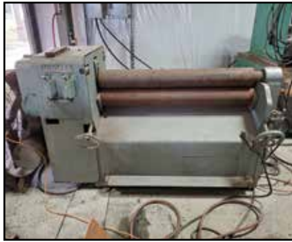
NIAGARA 6' x 3/16" Mild Steel Initial Pinch Bending Roll
