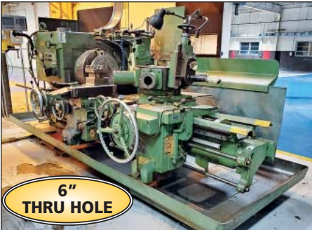
Warner & Swasey No. 3A Turret Lathe w/ 6" Thru Hole
