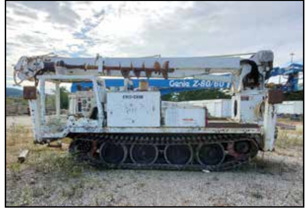
ALTEC DM47TR Digger Derrick Mounted on 2005 CENTRAL MINE CME-800 HDH Track All-Terrain Carrier
