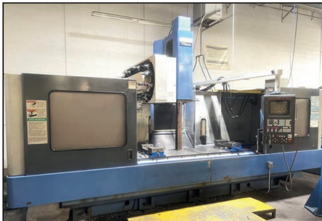
MAZAK MAZATECH MTV655/80 VERTICAL MACHINING CENTER
