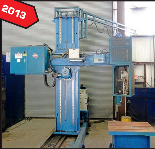
ARC SPECIALTIES ARC-6G BORE CLADDING SYSTEM
