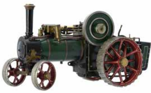
132 A well engineered ¾ inch scale model of a Bassett-Lowke live steam traction engine, having copper boiler with fittings, solid disc flywheel, single cylinder with trunk guide and displacement oiler fitted to side, steam safety valve and work and screw steering. The model finished in green and black paintwork with polished brass boiler bands and red spoked wheels fitted with strakes
