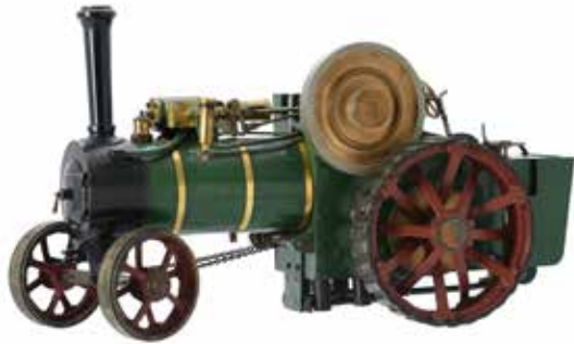
131 A well engineered ¾ inch scale model of a Bassett-Lowke live steam traction engine, the open crank with trunk guided to single cylinder having displacement oiler, safety valve, brake to back wheel and solid disc flywheel. The model finished in green and black paintwork with red straked wheels
