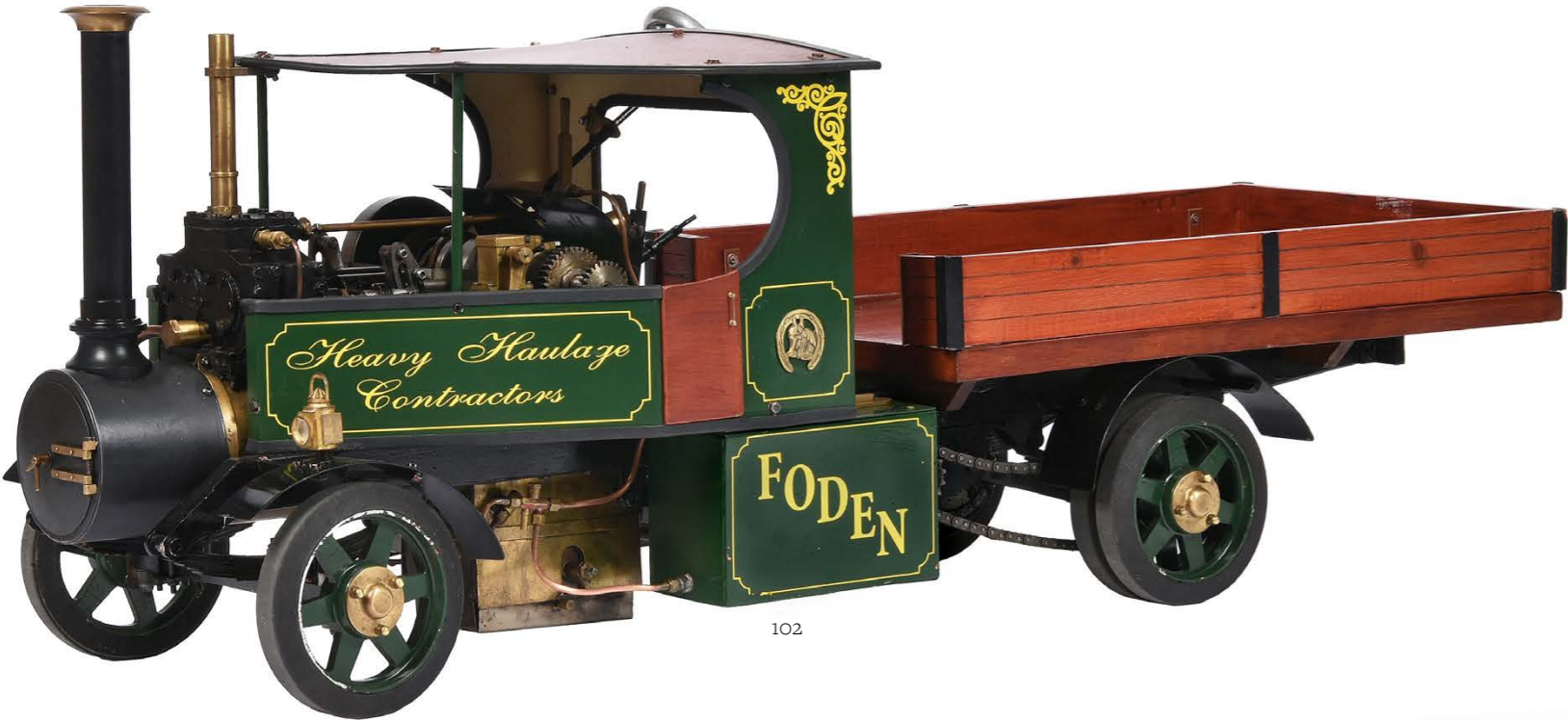
102 A well engineered 2 inch scale model of a Foden overtype open crank steam lorry, the copper silver soldered boiler with fittings including steam pressure gauge, water sight glass, associated copper piping and drain controls. The twin cylinder engine with trunk guides, Stephenson's reverse gear, ratchet oiler system, solid disc flywheel, chain drive to back axle. The model finished in green coachwork with sign writing 'Heavy Haulage Contractors' and 'Foden' to water tanks, fitted road lamps, wheels with rubber road tyres having polished brass hub caps and mud guards. The rear with planked lorry body. Overall length 130cm. Width 40cm. Height 45cm.
