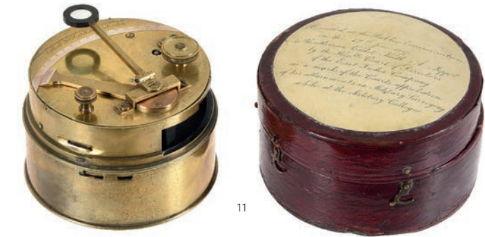
11 A VICTORIAN BRASS BOX SEXTANT PRESENTED TO GENTLEMAN CADET A. JOPP OF THE EAST INDIA COMPANY Elliott, London, circa 1857 circular top plate with screw for rack and pinion index mirror adjustment against a fine inset silver Vernier scale with magnification arm and signature Elliott, 268 High Holborn, London to outer margin, the circumference with sliding shutter for the pin hole sight, the instrument enclosed by a bayonet secured canister-shaped cover, the original blue velvet lined cylindrical red morocco covered box with brass presentation plaque to top finely engraved with the text Presented at the Public Examination, on the 12th June 1857, to Gentleman Cadet Keith A. Jopp, by the Hon'ble Court of Directors, of the East India Company, as a mark of the Courts approbation, of his attainments in Military Surveying, while at the Military College.
