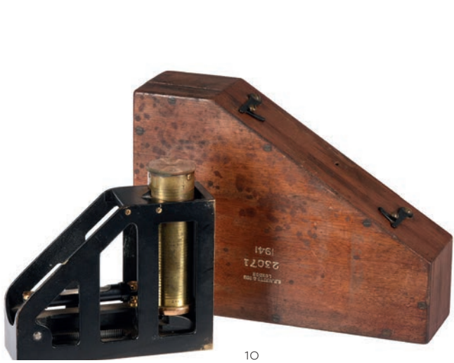
10 A JAPANNED AND LACQUERED BRASS INCLINOMETER E. R. Watts and Son, London, dated 1941 With pierced triangular frame enclosing spirit bubble scale with spring-loaded pivot at the open end, engaging with the underside of the brass fine-screw helical drum scale divided into tenths of a degree for reading against a pointer applied to the top plate of the tall end, the scale end plate engraved CLINOMETER, LARGE, E.R. WATTS & SON, LONDON, 1941, No. 23071 , in original shaped mahogany box stamped with repeat makers mark, serial number and date to lid.
