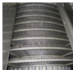
One of the Eurotek spiral freezers - 2 Available 16 & 17 tier
