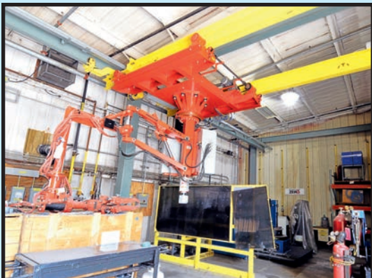
TARUS 1,500 LB. PART MANIPULATOR ON FREE STANDING CRANE SYSTEM
