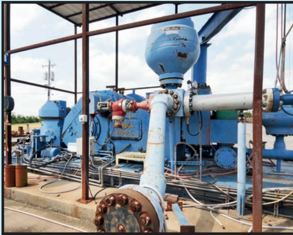
NATIONAL MDL. 850PT, 1,000 HP MUD PUMP/HYDROSTATIC TESTER
