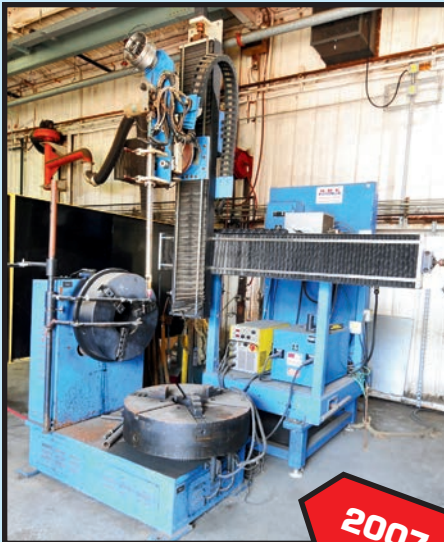
ARC SPECIALTIES MDL. ARC5-HG CIRCULAR OVERLAY SYSTEM
