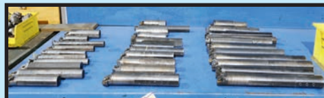
INDEXABLE CARBIDE BORING BARS
