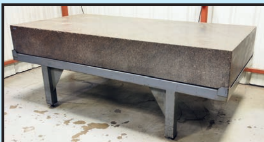
GRANITE SURFACE PLATE: 5' X 10' X 12" THICK
