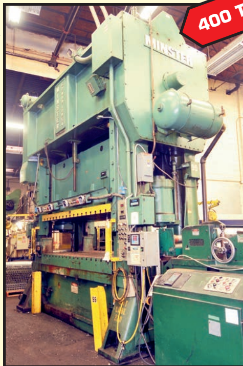
MINSTER E2-400-108-54 "HEVI-STAMPER" STRAIGHT SIDE ECCENTRIC GEARED PRESS
