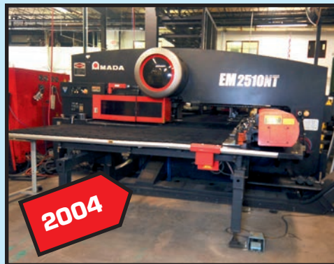
AMADA MDL. EM2510NT CNC TURRET PUNCH SYSTEM
