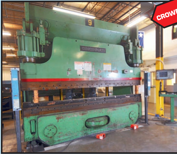
CINCINNATI 350 T. X 10' CNC PRESSBRAKE
