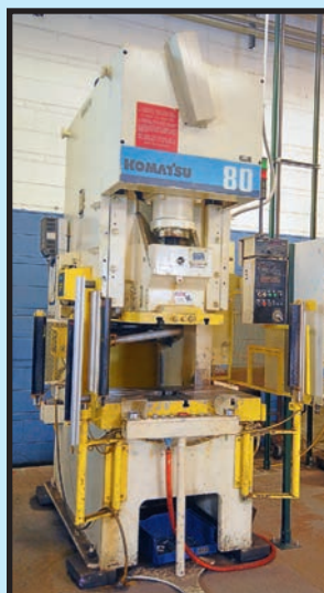
KOMATSU 88 T. SINGLE CRANK GAP PRESS
