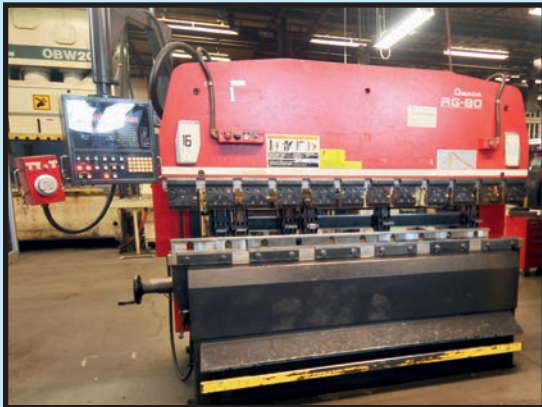
AMADA MDL. RG80 CNC PRESSBRAKE
