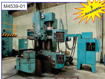
M4539-01 39" Froriep VTL, 4-jaw chuck, 39" UR, 5 pos. turret, side hd., 330 rpm, 75 hp, retrofit electrics
