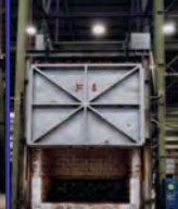
F8, 2200 Deg. F, 160" W x 118" H x 106" D, natural gas, 4 burners, fiber lined, Honeywell controls
