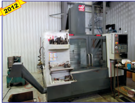
Haas VF-2 CNC VMC, new 2012 , 14" x 36" table, 40 taper, 8,000 rpm, 30 hp, 30" X / 16" Y / 20" Z, 4.0" - 24.0" spindle nose to table, 20 tool ATC
