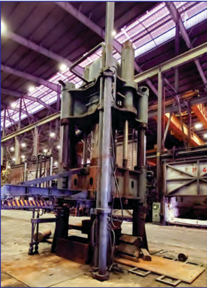
1400 Ton Lake Erie Press, 40" x 135" Bed with 96" Stroke, 36" x 93" (2) Station Die with 48" of Travel, 120", Daylight, 62" Stroke, 58" Btwn Uprights, 57" Window Width
