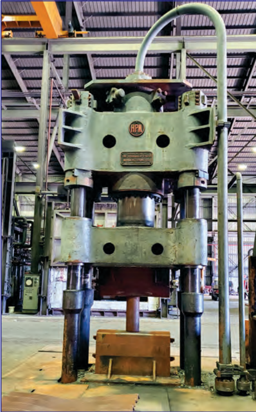
HPM 1000 Ton Forging Press, 48" x 66" Bed, 48" x 67" Ram, 98" Daylight, 34" Stroke, 69" Between Uprights
