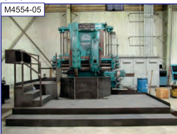
M4554-05 54" Bullard Cutmaster Hi-Column VTL, 4-jaw chuck, 68" UR (24" extra height), L ram, R turret, side hd., 160 rpm, 50 hp, oper. platform
