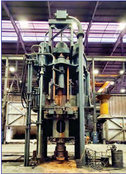
2500 Ton Babcock & Wilcox Preforming Press, 32" x 157" Bed with 57" Travel, 35" x 63" Sliding Ram with 8" Travel, 114" Daylight, 52" Stroke, 76" Btwn Uprights, 42" Window Width, FSI PLC Controlled
