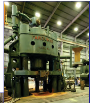
2014, Babcock & Wilcox 3300 Ton Open Die Forging Press, 84" x 210" Sliding Bed with 116" of Trvl, 42" x 88" Ram, 240" Daylight, 120" Stroke, 54" Between Uprights, 112" Window Width
