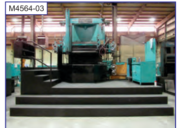
M4564-03 64" Bullard Hi-Column VTL, 4-jaw chuck, 80" UR, L ram, R turret, side hd., 100 rpm, 75 hp, oper. platform
