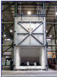
S2, 2200 Deg. F Epcon Furnace, 151" W x 141" H x 132" D, natural gas, 4 burners, fiber lined, Honeywell controls
