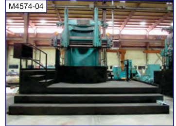
M4574-04 74" Bullard Cutmaster Hi-Column VTL, face plate w/4 jaws, 84" UR, L ram, R ram, side hd., 97 rpm, 50 hp, oper. platform
