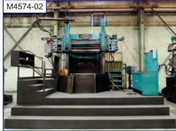
M4574-02 74" Bullard Cutmaster VTL, face plate w/4 jaws, 64" UR, L ram w/ turret, R ram, 90 rpm, 60 hp, oper. platform
