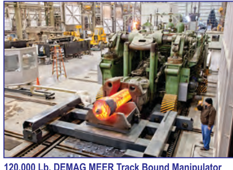
120,000 Lb. DEMAG MEER Track Bound Manipulator with hot forging billet
