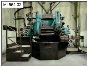
M4554-02 54" Bullard Cutmaster VTL, 4-jaw chuck, 44" UR, L ram w/ tracer, R turret, side hd., 160 rpm, 60 hp, oper. platform
