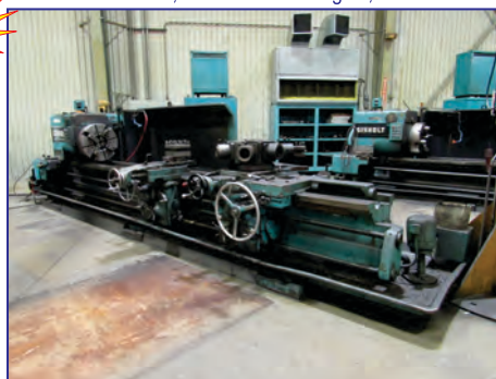
Gisholt 3L Turret Lathe , 24" 4-jaw chuck, 6" thru-hole, 120" bed length, hex tool turret
