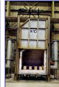
W10, 1850 Deg. F, 98" W x 68" H x 82" D, natural gas, 2 burners, fiber lined, Honeywell controls
