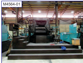
M4564-01 64" Bullard VTL, 4-jaw chuck, 54" UR, L ram w/ turret, R turret, side hd., 100 rpm, 75 hp, oper. platform
