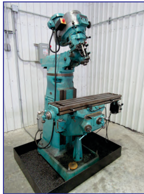
Bridgeport Series I Vertical Mill , 9" x 42" table, 2 hp, pwr cross feed, lube
