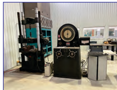
Southwark-Emery Compression Tester, 120,000 lbs. comp. cap., 34" max. part length
