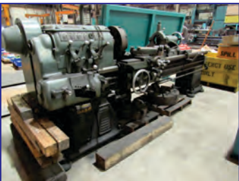
20" x 72" Monarch Engine Lathe , 20" swing, 72" ctrs, 15" 4-jaw chuck, 6" steady rest, tailstock, taper attach.
