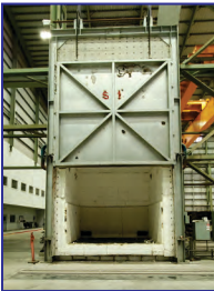
S1, 2200 Deg. F Epcon Furnace, 151" W x 141" H x 132" D, natural gas, 4 burners, fiber lined, Honeywell controls
