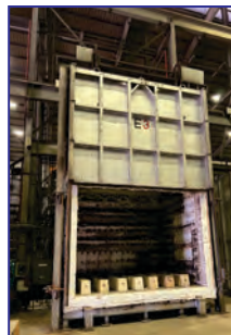
E3, 2100 Deg. F, 170" W x 117" H x 140" D, natural gas, 6 burners, fiber lined, Honeywell controls
