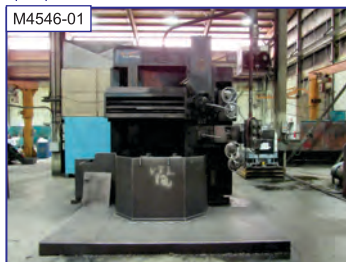
M4546-01 46" Bullard Cutmaster Model 75 VTL, 4-jaw chuck, 46" UR, L ram w/ tracer, R turret, side hd., 40 hp, oper. platform
