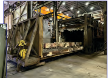
E6, 2400 Deg. F Custom Built Car Bottom Furnace, 135" W x 80" H x 320" D, natural gas fired, 14 burners, fiber lined, Honeywell controls
