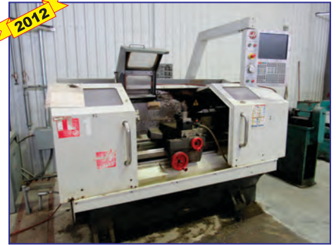
Haas TL-1 CNC Lathe, new 2012 , 20" swing over apron, 11" over slide, 30" max. cut length, 8" X / 30" Z, 1800 rpm, 10 hp, 6" 4-jaw chuck, 2.3" spindle bore, tailstock
