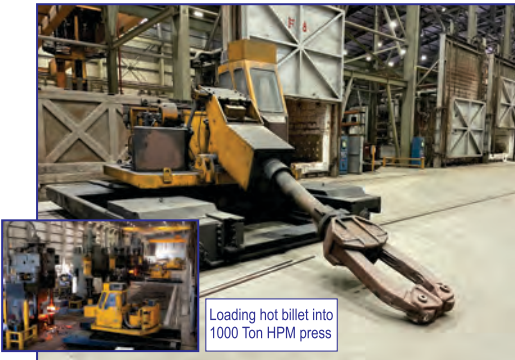
8,000 Lb. Columbiana Rail Bound Manipulator, 216" rail span, 242" width, 120" btwn axles, 168" length, 17 ft. reach from rotation ctr, 12 ft. max. ext. reach, 108" trvl in/out, 72" max. tong ht., updated electronics
