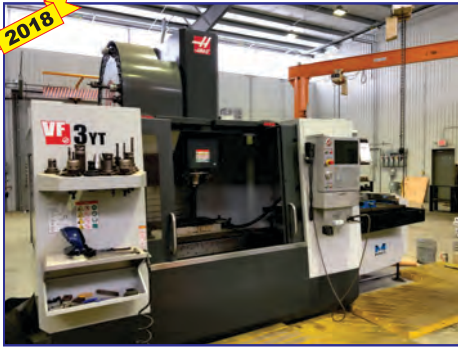
Haas VF-3YT CNC VMC, new 2018 , 24" x 54" table, 50 taper, 10,000 rpm, 30 hp, 40" X / 26" Y / 25" Z, 7.9" - 32.9" spindle nose to table, 30 tool ATC, Midaco pallet changer
