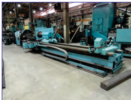
VDF Wohlenberg Type E1120 Lathe , 46" swing, 32" over slide, 39" face plate w/ 4 jaws, 3" hole, 276" ctrs, 315 rpm, roller steady, chuck on tailstock, motorized tailstock
