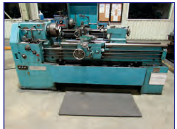
16" x 60" Summit Gap Bed Engine Lathe , 16" swing, 22" in gap, 60" ctrs, 3-jaw chuck, 1500 rpm, Aloris tool holder, tailstock, taper attach.,
