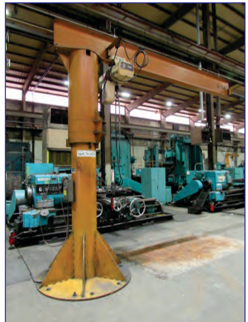
2 Ton Pedestal Jib Cranes , approx. 20 available, most with 2 ton Coffing hoists
