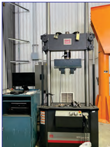
MTS 370.50 Fatigue Tester, 500 kN force, 6" actuator stroke, 13" - 78" specimen length
