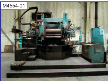
M4554-01 54" Bullard Cutmaster VTL, face plate w/4 jaws, L ram w/ tracer, R turret, side hd., 120 rpm, 50 hp, oper. platform
