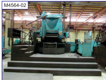
M4564-02 64" Bullard Hi-Column VTL, face plate w/4 jaws, 78" UR, L ram w/ tracer, R turret, 133 rpm, 60 hp, oper. platform
