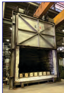
E5, 2100 Deg. F, 165" W x 118" H x 140" D, natural gas, 6 burners, fiber lined, Honeywell controls
