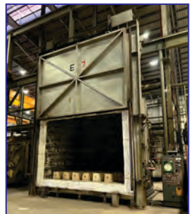
E7, 2100 Deg. F, 165" W x 117" H x 138" D, natural gas, 6 burners, fiber lined, Honeywell controls
