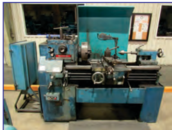
16" x 36" LeBlond Engine Lathe , 16" swing, 36" ctrs, 12" 3-jaw chuck Aloris tool holder, tailstock, taper attach., work light
