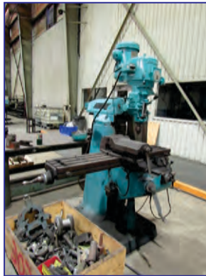
Bridgeport Series I Vertical Mill , 9" x 49" table, 2 hp, pwr cross feed, var. speed head
