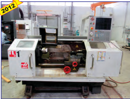
Haas TL-1 CNC Lathe, new 2012 , 20" swing over apron, 11" over slide, 30" max. cut length, 8" X / 30" Z, 1800 rpm, 10 hp, 6" 4-jaw chuck, 2.3" spindle bore, tailstock
