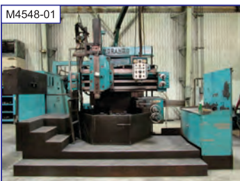
M4548-01 48" Morando VTL, 4-jaw chuck, 42" UR, ram w/ tracer, side hd., 300 rpm, 70 hp, oper. platform
