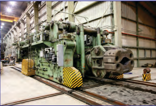
120,000 Lb. DEMAG MEER Track Bound Manipulator, TYP 600 KNM, 126" rail span, 228" width, 37 ft. overall length (w/ grip), 202" wheel base, 16 ft. overall ht. with piping
