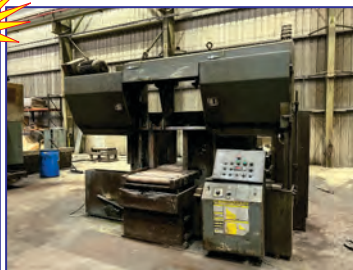
Hyd-Mech H-22A Horizontal Bandsaw, 24" x 24" cap., bundle attach., power feed
