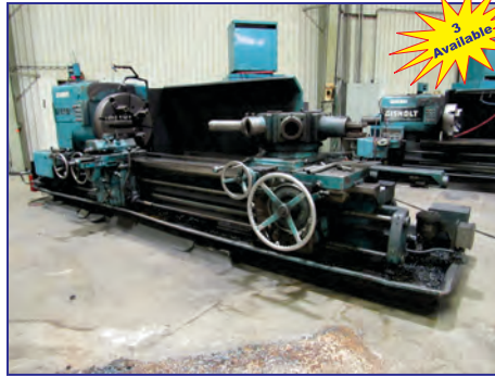
Gisholt 5L Turret Lathes , 28" to 32" 4-jaw chucks, 9.75" to 12.75" thru-holes, 84" to 96" bed lengths, hex tool turrets
