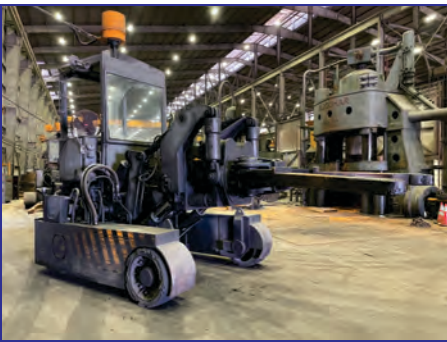
8,000 Lb. Glama Trackless Manipulator, 100" width, 98" whl base, 132" length (w/o tongs), 96" tong length, 96" reach, 72" max. tong ht., 62" max. tong opening
