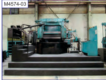
M4574-03 74" Bullard Cutmaster VTL, face plate w/4 jaws, 64" UR, L ram w/ turret, R ram, side hd., 90 rpm, 60 hp, oper. platform
