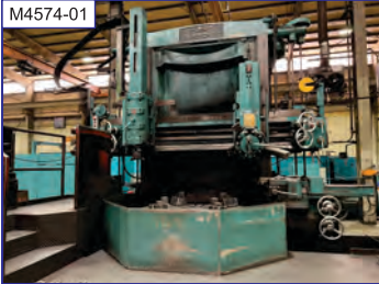
M4574-01 74" Bullard Cutmaster Hi-Column VTL, face plate w/4 jaws, 86" UR, L ram w/ tracer, R turret, side hd., 120 rpm, 125 hp, oper. platform
