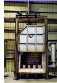
W8, 1850 Deg. F, 97" W x 58" H x 86" D, natural gas, 2 burners, fiber lined, Honeywell controls
