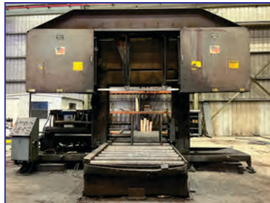
HEM DC-6060 Horizontal Bandsaw, new 1997, 60" x 60" cap., 2-5/8" blade, coolant, power feed, new controls 2014
