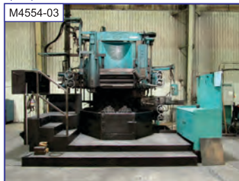
M4554-03 54" Bullard Cutmaster Hi-Column VTL, face plate w/4 jaws, 68" UR (24" extra height), L ram w/ tracer, R turret, side hd., 160 rpm, 50 hp, oper. platform
