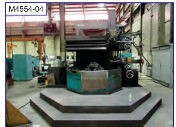
M4554-04 54" Bullard Cutmaster VTL, face plate w/4 jaws, 44" UR, R turret, side hd., 160 rpm, 30 hp, oper. platform
