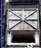
F6, 2200 Deg. F, 160" W x 118" H x 106" D, natural gas, 4 burners, fiber lined, Honeywell controls
