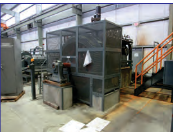
1400 Ton Lake Erie Press, 40" x 135" Bed with 96" Stroke, 36" x 93" (2) Station Die with 48" of Travel, 120", Daylight, 62" Stroke, 58" Btwn Uprights, 57" Window Width
