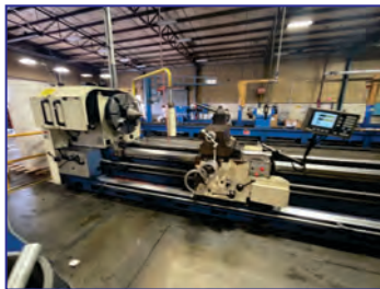
42" x 320" Summit Lathe with 9" Bore
