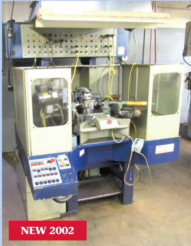
WIRTH & GRAFFAT C126 Rotary Transfer Machine
