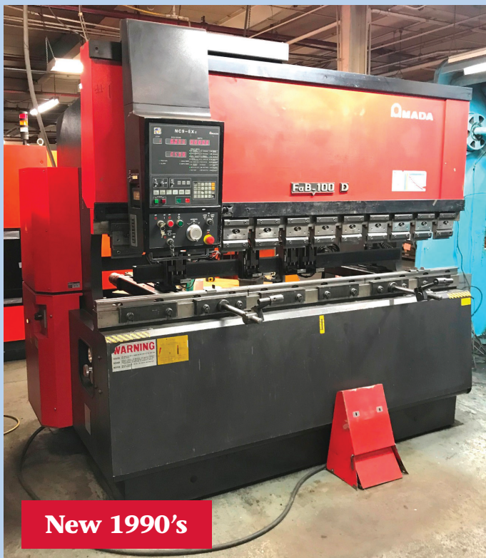
Amada Model FBD-1025E 8' x 100-Ton 3-Axis CNC Press Brake
