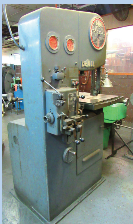
DoAll Model 1612-3 16" Vertical Hydraulic Band Saw
