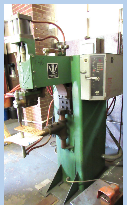
Lors Model 150AP 50 KVA Press-Type Welder with Interlock Model 105 Microprocessor Control
