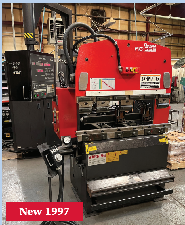
Amada Model RG-35s 50" x 38-Ton 3-Axis CNC Press Brake
