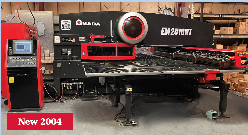
Amada Model EM2510NT 22-Ton CNC Turret Punch with Fanuc AMCF-F Control
