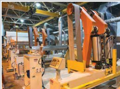
View of 84" AMD Slitter Rewinder W/ Belt Driven Unwinds
