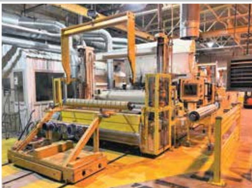
View of 84" AMD Slitter Rewinder W/ Belt Driven Unwinds
