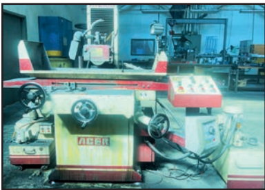
ACER 1020AH AUTOMATIC SURFACE GRINDER
