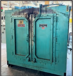
TRENT 30 KW ELECTRIC BATCH OVEN
