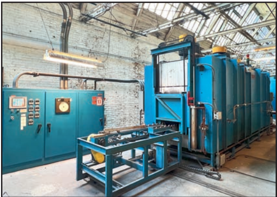
WISCONSIN OVEN COMBFLOW E10/3Z ELECTRIC HEAT TREAT OVEN
