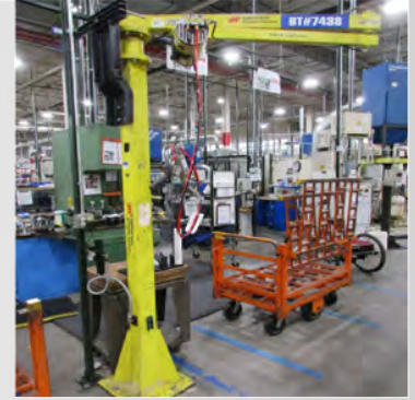
INGERSOLL RAND 720 150 LB. FREE-STANDING ARTICULATING JIB CRANE
