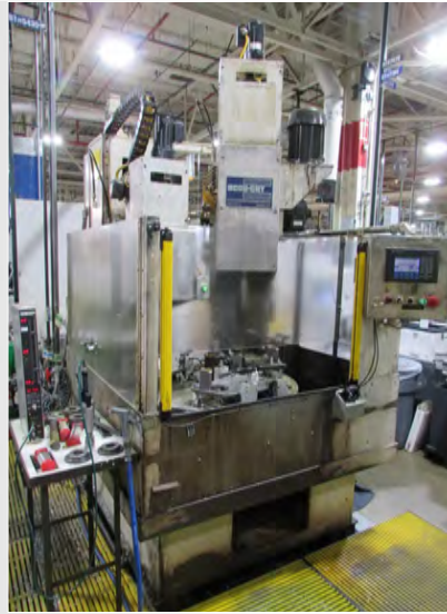
ACCU-CUT DIAMOND TOOL 2X1SMCRIG 3-STATION VERTICAL BORE SIZING HONE
