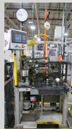
SHOP-BUILT ASSEMBLY STATION WITH INSERTION PRESS
