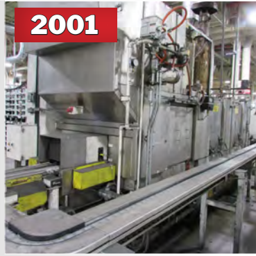
2001 CAE RANSOHOFF 4066 3-STAGE AUTOMATIC CONVEYOR PARTS WASHER
