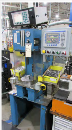
NEFF 12.4 TON HYDRAULIC GAP FRAME PRESS
