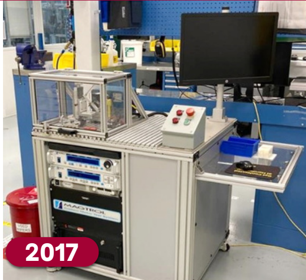
(2) MAGTROL TESTING STATIONS WITH DYNAMOMETERS, ELECTRONICS & SOFTWARE
