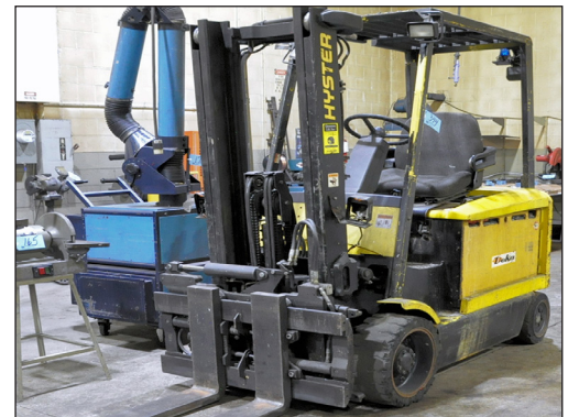
Hyster Model E65XM, 6500-Lbs. x 126" Lift Capacity Sit Down Ride On Electric Fork Lift Truck
