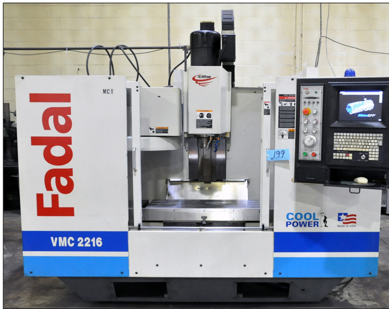
Fadal Model VMC-2216, CNC Vertical Machining Center, Box ways, 32MP Control, 21 ATC, Gibbs Cam, (2002)
