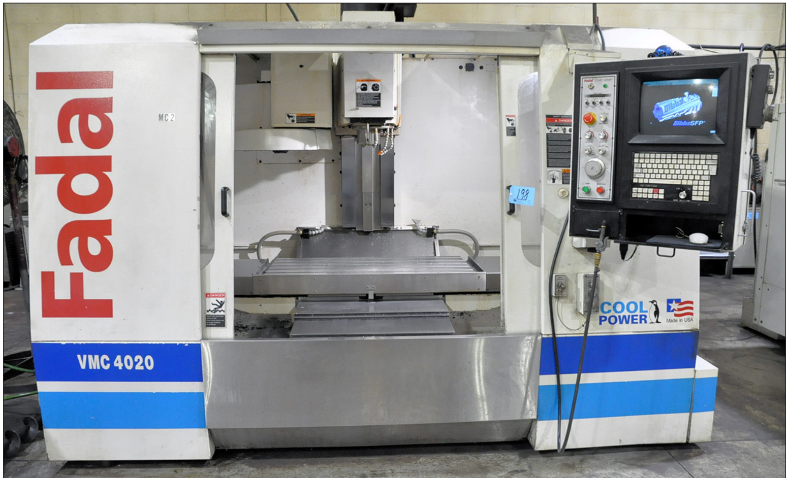
Fadal Model VMC 4020, CNC Vertical Machining Center, Box ways, 32MP Control, 21 ATC, Gibbs Cam (2000)
