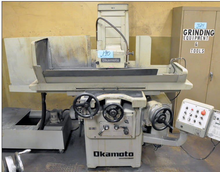
Okamoto 820A, Fully Automatic Surface Grinder, Incremental Downfeed, (1990)
