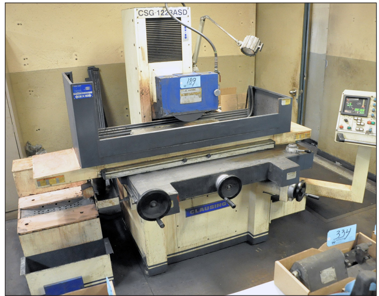
Clausing 12" x 28", Fully Automatic Surface Grinder, Incremental Downfeed, (1998)
