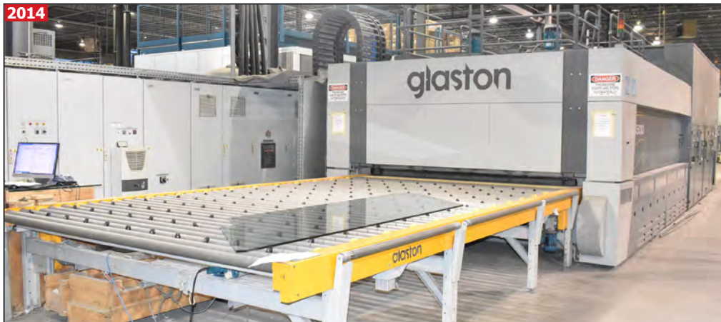
GLASTON-TAMGLASS FC-500-2848-380L tempering furnace
