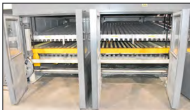
Interior view of GLASTON-TAMGLASS tempering furnace
