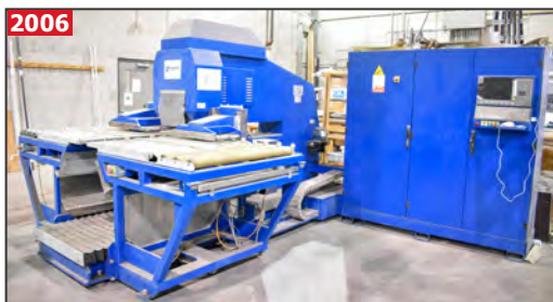
FORVET FC 16M1250 CNC twin head drilling & milling machine
