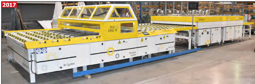
GOLD GLASS TECHNOLOGIES M.R.C 2850-M CNC flat glass paint line & GOLD GLASS TECHNOLOGIES GD7000 paint drying machine
