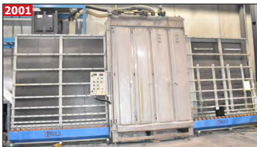
TRIULZI VTIS.SP.2600.4.2.2 vertical glass washer
