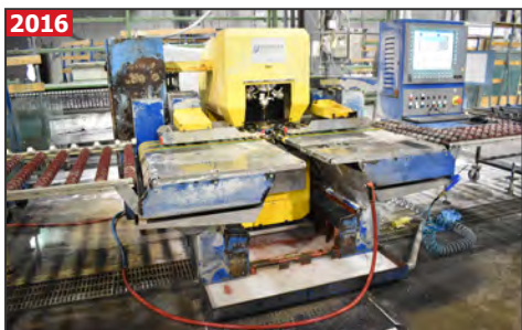
FORVET FRANCESCA 1250 H.O. CNC twin head drilling and milling machine
