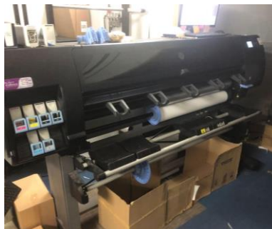
HP DesignJet Z6600 60" large format printer
