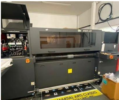
EFI H1625LED wide format industrial 1.6m mid-level production printer
