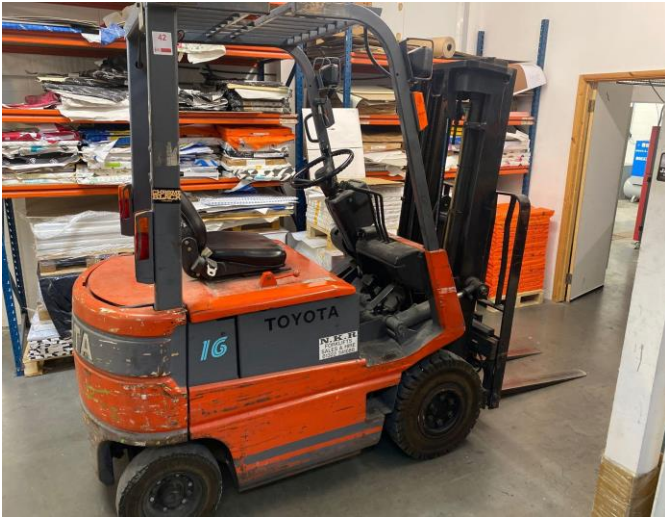
Toyota FBM 16 electric side shift forklift truck
