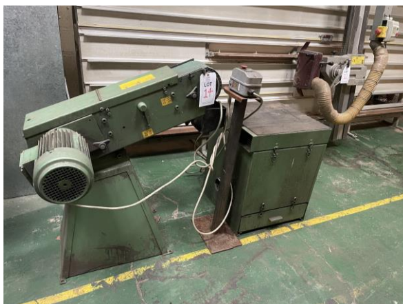
BM 1000 inclined belt sander with dust collection unit
