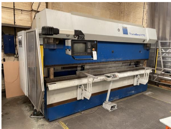
Trumpf Trumabend V170 hydraulic press brake (2000)
