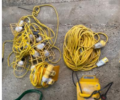
Festoon lighting & Transformers
