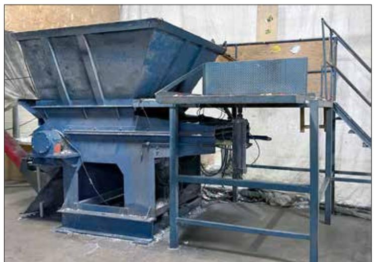
VECOPLAN RETECH Grinder Shredder
