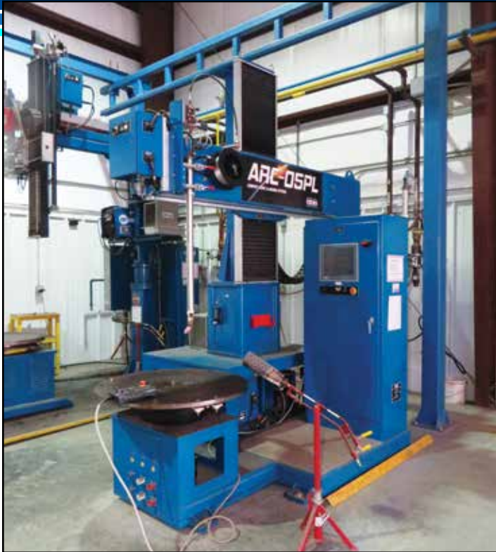
ARC SPECIALTIES ARC-05PL 6'x 6' WELDING MANIPULATOR BORE CLADDING AND INCONEL WELDING SYSTEM
