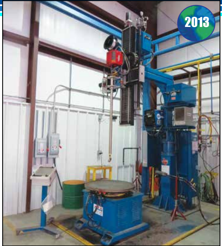
ARC SPECIALTIES ARC-5P+ WELDING MANIPULATOR BORE CLADDING & INCONEL WELDING SYSTEM
