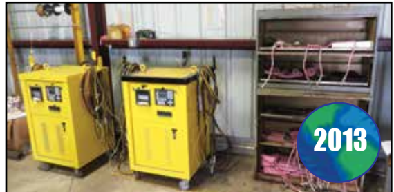
(2) PDS BARTECH PCE-30 HEAT TREATING CONSOLES
