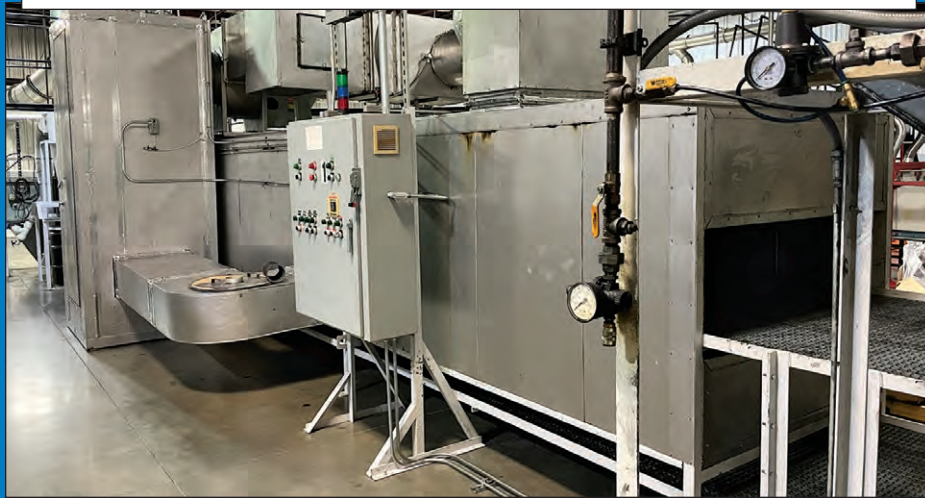
48" Cusi Oven, Modular Panel, Approx. 40' Tunnel
