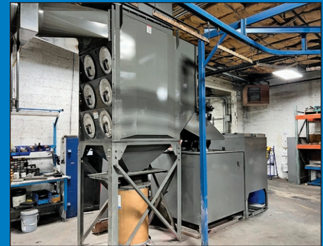
30 HP Torit Model DF03-12(8K) Six Cartridge Dust Collector
