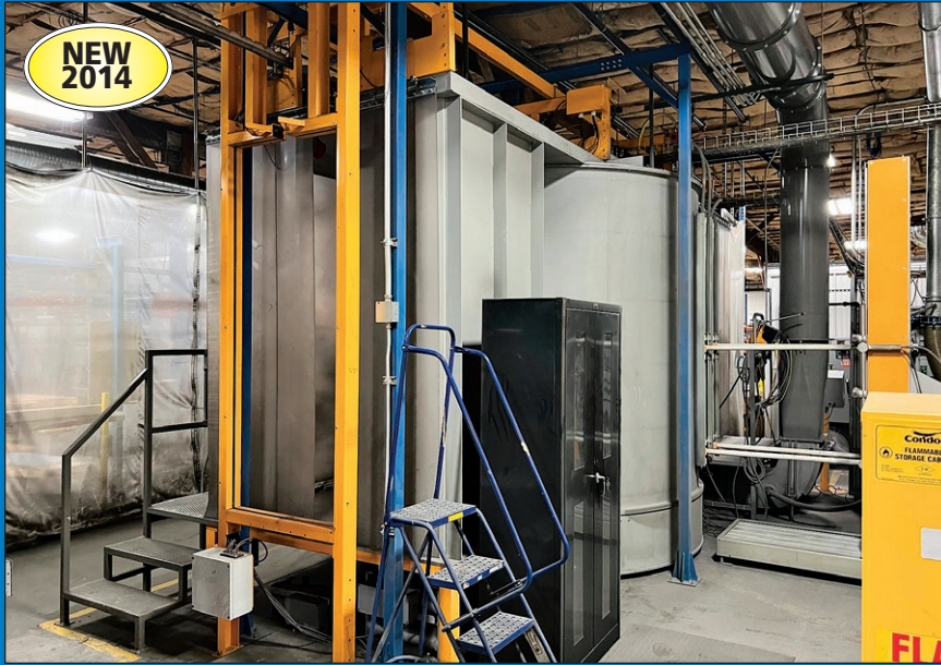
ITW Gema Eight-Gun Automatic Pass-Thru Powder Coat Booth; 31" x 80" Window (2014)
