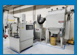
Guyson RXS900 Multi-Station Blast System w/ Dust Collector
