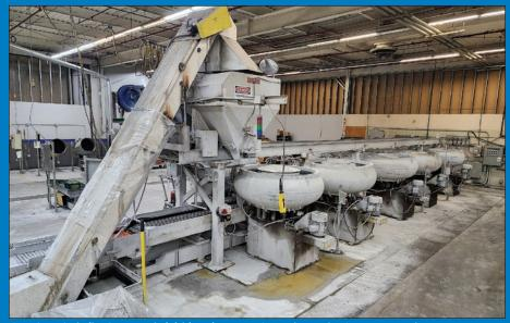
(2) Automated Vibratory Bowl Finishing Lines w/ (16) Bowls, Loader Conveyors and Hoppers
