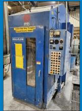
Sinto Roll-Flow EVF-08R Centrifugal Disc Finisher
