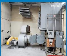
40-HP Dust Hog 16-Cartridge Dust Collector
