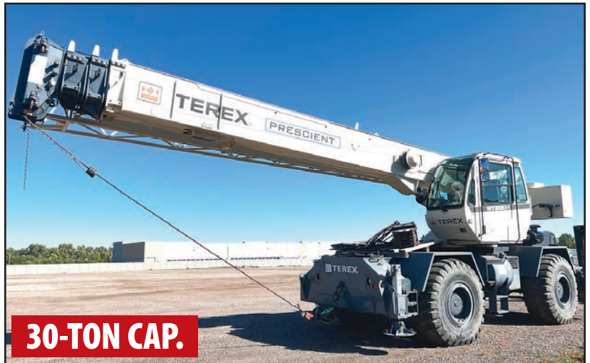
TEREX TR230-1 30-TON MOBILE CRANE
