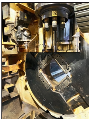
MAZAK WORK ENVELOPE, BEVEL HEAD, TAPPING UNIT
